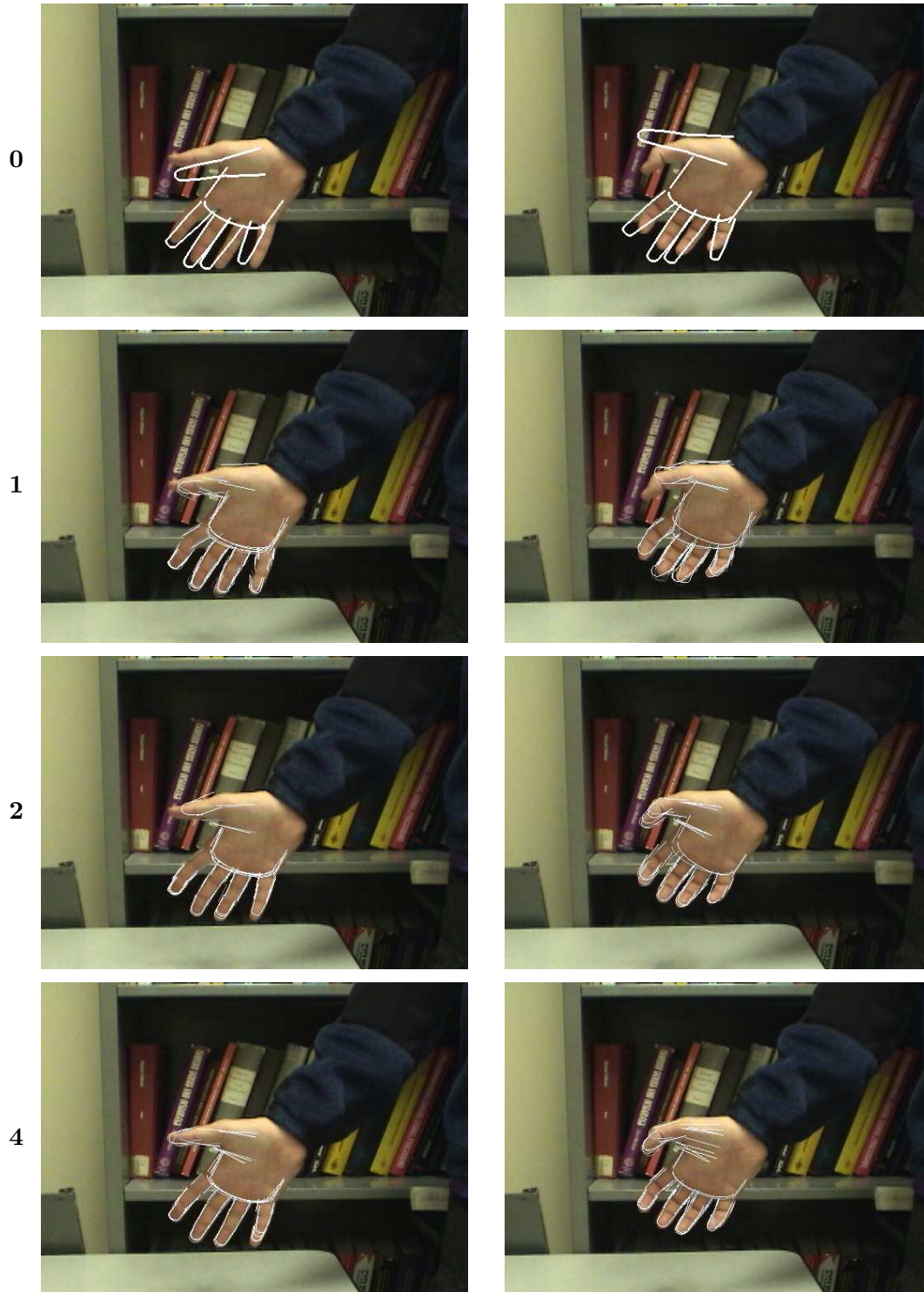
Figure 4.8. Two examples (columns) in which NBP iteratively refines coarse initial hand pose estimates. We show projections of the estimated 3D hand pose following 1, 2, and 4 iterations of the sequential message schedule illustrated in Fig. 4.7.
