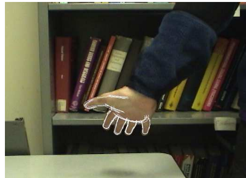
Figure 4.10. Four frames from a video sequence showing extrema of the hand's rigid motion, and projections of the NBP tracker's 3D pose estimates.
