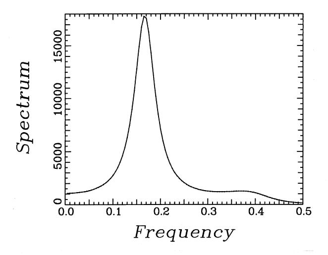
Figure 5.8: Plot of the estimated power spectrum in Example 5.4.1 when estimates of the covariance function are computed over a disk of radius 20 m given the data over a disk of radius 30 m and with N=5.
