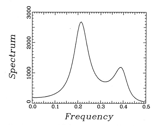
Figure 5.7: Plot of the estimated power spectrum in Example 5.4.1 when estimates of the covariance function are computed over a disk of radius 20 m given the data over a disk of radius 100 m and with N=5.
