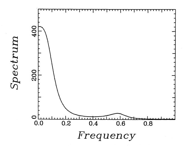
Figure 5.15: Plot of the estimated power spectrum in Example 5.4.3 when exact covariance data is given over a disk of radius 20 m and with A=1 and N=10.
