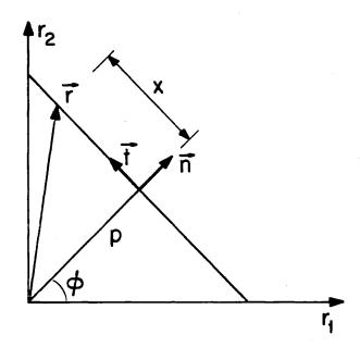
Figure 6.1: Coordinate system associated to the line L.
