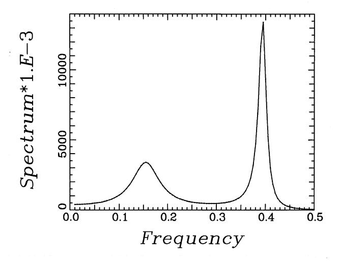
Figure 5.9: Plot of the estimated power spectrum in Example 5.4.1 when estimates of the covariance function are computed over a disk of radius 20 m given the data over a disk of radius 100 m and when  $P = 10^{-3}$  Watt.m<sup>2</sup> and N = 5.
