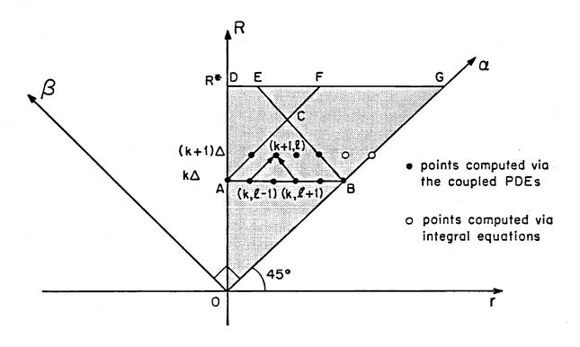
Figure 5.1: Discretization scheme and numerical implementation of the recursions for  $g_n(R,r)$ .
