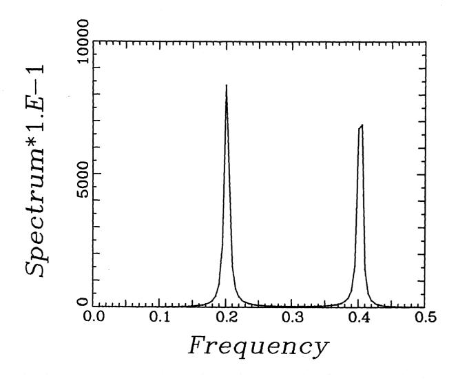
Figure 5.3: Plot of the estimated power spectrum in Example 5.4.1 when exact covariance data is given over a disk of radius 20 m and with N=1.
