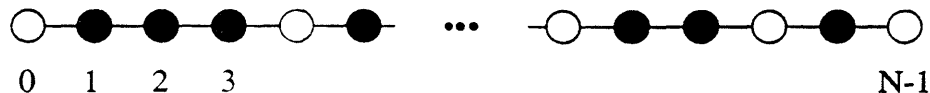
Figure 3-9: A sample path of a 1-D Ising process is shown. The process can take on two states or spins , represented above by empty and filled circles.
