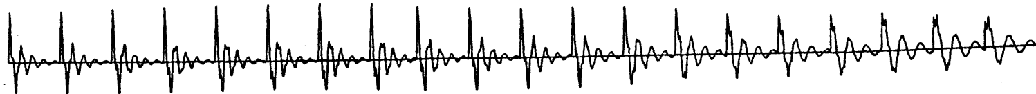
Figure 4.7c Reponse of 6-2 Autocorrelation Power Filter (with windowing the original data)
