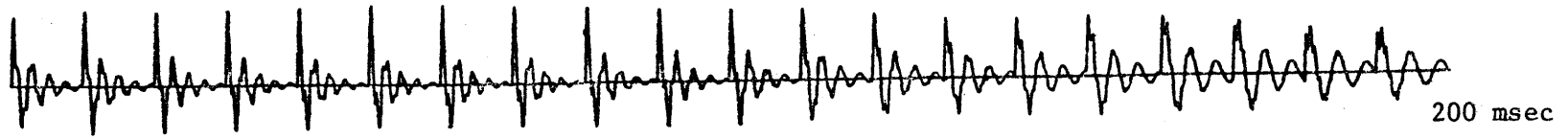
Figure 4.7a Response of 6-2 Covariance Fourier Filter (without windowing the original data)
