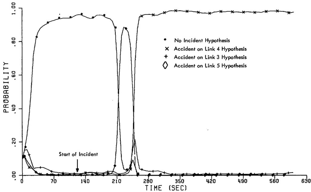
Fig. 5. MM probability plot. Accident on link 4; nominal flow=1000 cars/h/lane; aggregate measurements from microscopic simulation.
