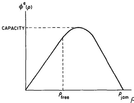
Fig. 2. The fundamental diagram of traffic.
