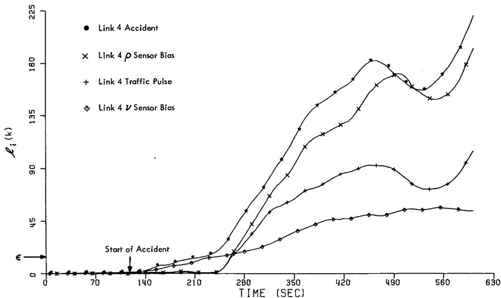
Fig. 6. GLR,  $l_i(k)$ : Accident on link 4; nominal flow=1000 cars/h/lane; aggregate measurements from microscopic simulation.
