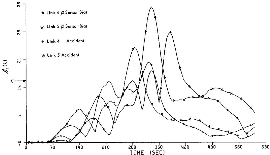
Fig. 8. GLR,  $l_i(k)$ : No accident, two slowly moving vehicles; nominal flow=1600 cars/h/lane; aggregate measurements from microscopic simulation.
