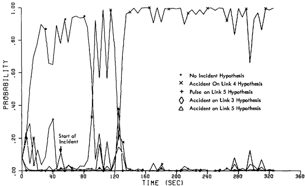
Fig. 3. MM probability plot. Accident on link 4, nominal flow=1000 cars/h/lane; aggregate model simulation.
