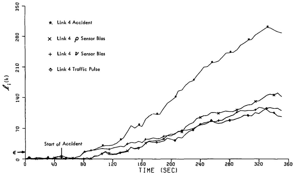
Fig. 4. GLR,  $l_i(k)$ : Link 4 accident; nominal flow=1000 cars/h/lane; aggregate model simulation.
