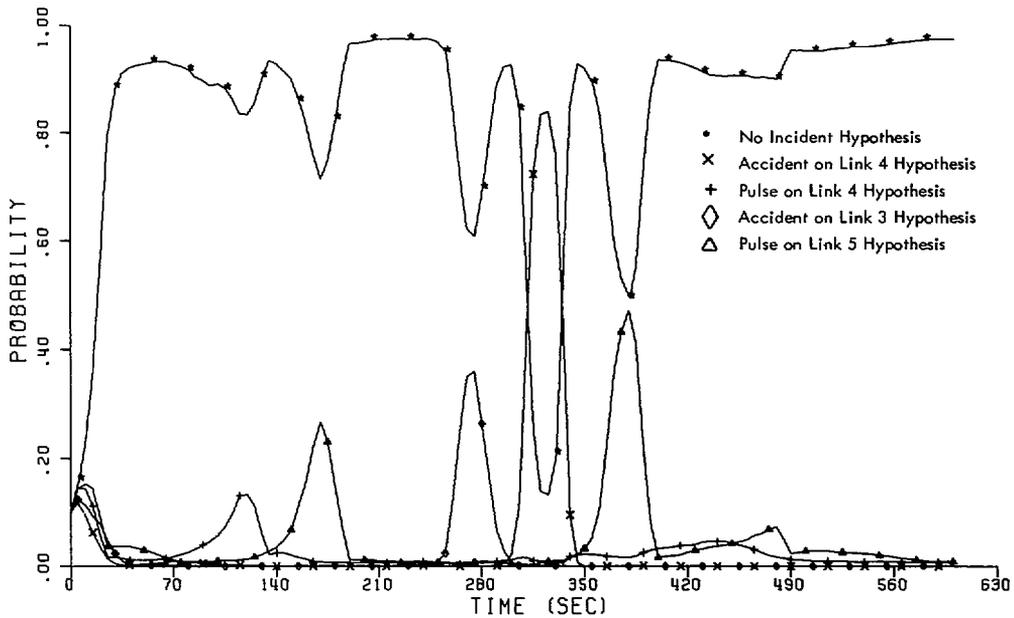
Fig. 7. MM probability plot. No accident, two slowly moving vehicles; nominal flow=1000 cars/h/lane; aggregate measurements from microscopic simulation.
