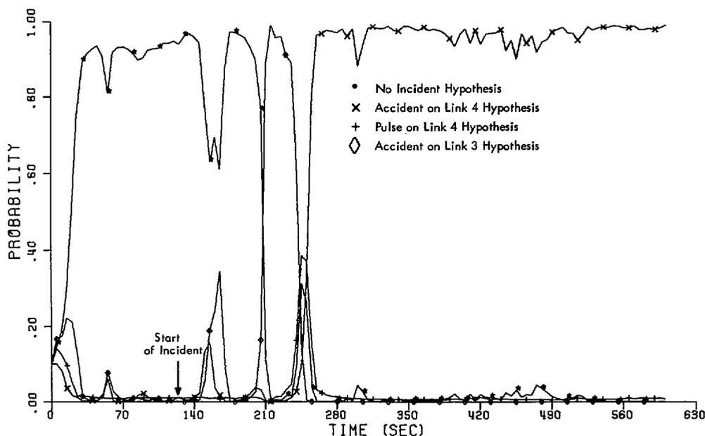
Fig. 9. MM probability plot. Accident on link 4; nominal flow=1000 cars/h/lane; presence detector data.
