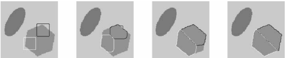
FIG. 5. The sensitivity of the region competition flow (18) to initial contour placement is shown by placing two contours near the same object. Both contours flow into the green object.
