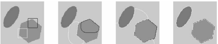
FIG. 7. The coupled ternary flows (13)–(14) do not allow both contours to flow into the green object. As one curve moves in, the other is forced out, even before they touch each other.
