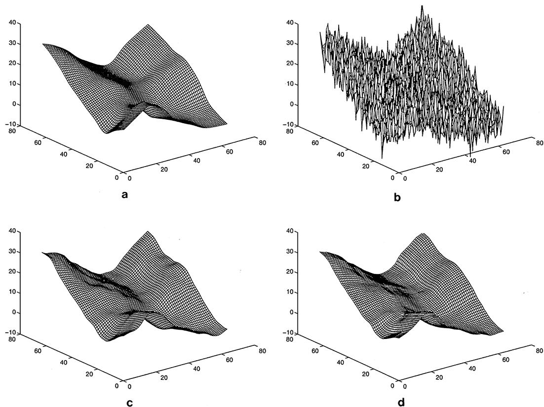
**FIG. 8.** Dense measurement reconstruction example: a surface is reconstructed based on dense measurements with 5 cm Gaussian noise. The multiscale and multigrid approaches involve the same number of computations.  $B_s = 80$ ,  $B_g = 0.4$ ,  $\mathcal{O} = (12, 6, 4, 3, 0, 0, 0)$ . (a) Original surface to be estimated; (b) original surface plus noise; (c) multigrid construction; (d) multiscale reconstruction.
