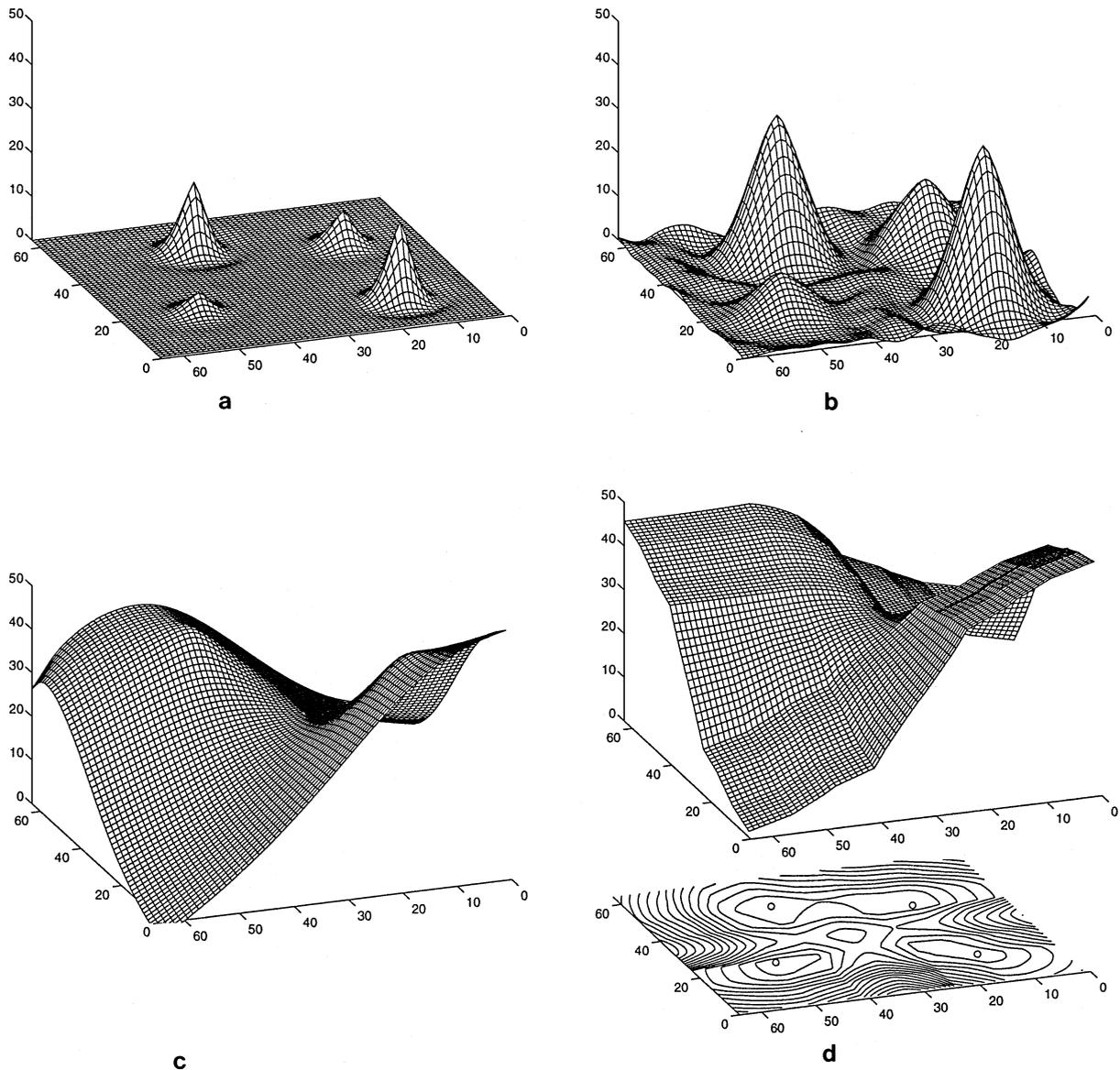
**FIG. 12.** Sparse measurement reconstructions using the same four methods of Fig. 11, but using one fourth of the computational effort in each case. Each minimum of the error surface in (d) is marked by an “o.”  $B_s = 80$ ,  $B_g = 0.05$ ,  $\mathcal{O} = (16, 10, 7, 0, 0, 0, 0)$ . (a) Gauss–Seidel reconstruction; (b) conjugate–gradient reconstruction; (c) multigrid; (d) multiscale.
