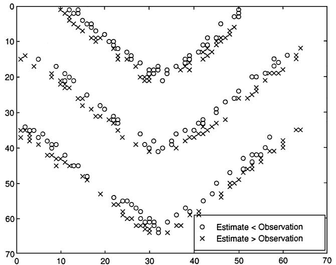
**FIG. 19.** Distribution of those measurement residuals, in excess of  $3\sigma$ , from the estimates based on *no* knowledge of the discontinuity locations, with the same measurements as in Fig. 18.  $B_s = 20$ ,  $B_g = 0.2$ ,  $\mathcal{O} = (26, 19, 14, 9, 0, 0, 0, 0)$ .
