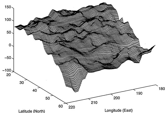
**FIG. 20.** A plot of the estimated ocean height, viewed from the north-east.  $B_s = 35\text{cm}$ ,  $B_g = 0.5$ ,  $\mathcal{O} = (16, 10, 5, 3, 1, 1, 0, 0)$ .
