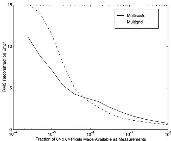
**FIG. 9.** RMS error in surface estimation using multiscale and multigrid methods as a function of the proportion of noisy measurements retained.
