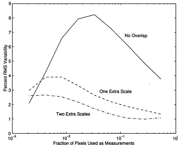
**FIG. 15.** Shift-variability of the multiscale estimates over random choices of the tree origin, as a function of the fraction of surface measurements. The vertical axis measures the RMS variability of the surface, normalized by the RMS value of the “truth” surface.
