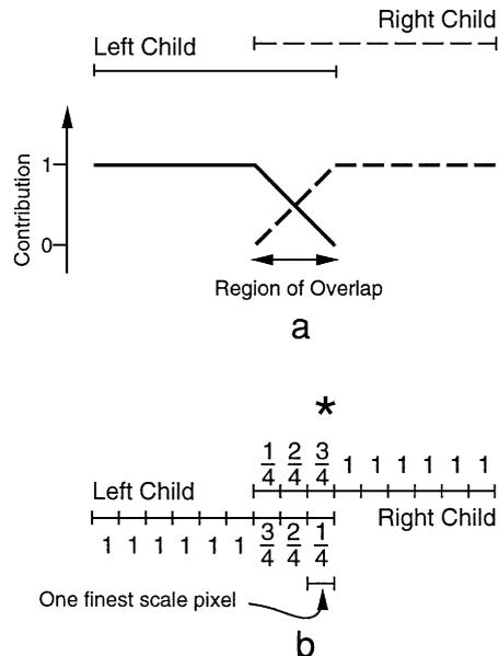
**FIG. 7.** Two overlapping nodes: the set of relative contributions to each finest scale pixel must sum to one. The contributions are tapered linearly over the region of overlap. (a) Tapering pictorially; (b) a specific example for two nodes which overlap by three pixels.
