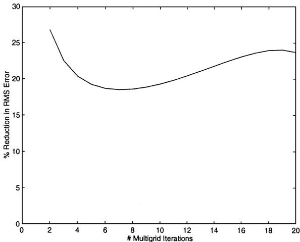
**FIG. 14.** Percent reduction in RMS error from just using  $i$  iterations of multigrid to computing estimates using the multiscale approach and using these estimates as the initial values for additional by multigrid iterations such that the total computation is equal to that of  $i$  multigrid iterations. The horizontal axis measures  $i$ .
