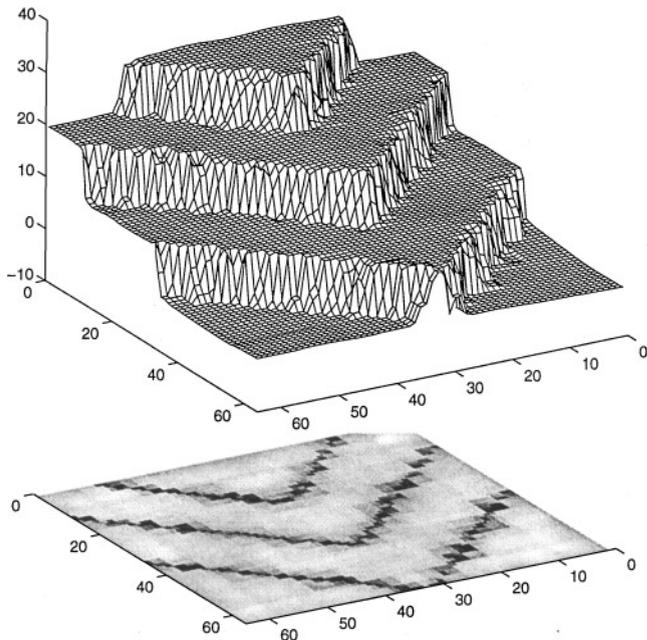
**FIG. 18.** Reconstruction of the surface of Fig. 16 and associated estimation error variances based on a knowledge of discontinuity locations and a sampling, at random, of one-third of the surface pixels having unit variance Gaussian noise added. The lower half of the figure plots the estimation error variances; darker regions represent greater uncertainty.  $B_s = 20$ ,  $B_g = 0.2$ ,  $\mathcal{O} = (26, 19, 14, 9, 0, 0, 0, 0)$ .
