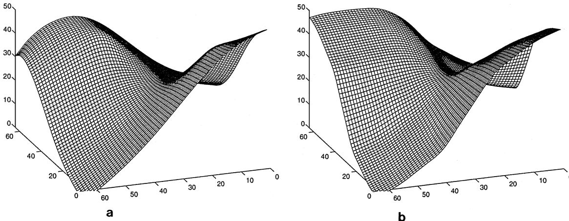
**FIG. 13.** Surface reconstructions computed by applying one multigrid iteration to the two surfaces Figs. 12c and 12d.  $B_s = 80$ ,  $B_g = 0.05$ ,  $\mathcal{O} = (16, 10, 7, 0, 0, 0, 0)$ . (a) Multigrid; (b) multiscale + multigrid.
