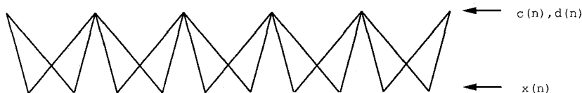
Fig. 2. Transformation of a 10-point sequence x(n) into 6-point scaling coefficients c(n) and its 6-point wavelet coefficients d(n) .
